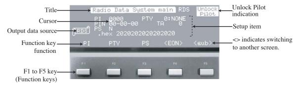
Fig. 2-4 Radio Data System main RDS Screen
